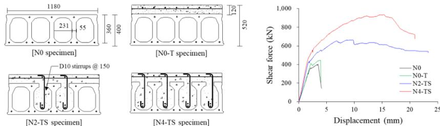
Fig. 1 Comparison of shear behavior of HCSs with and without strengthening
